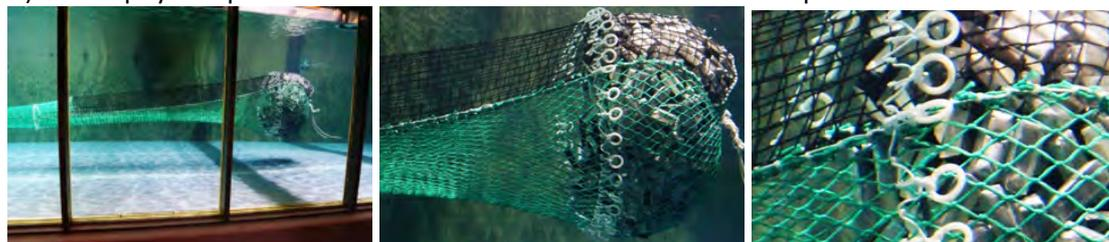
Photographs of Bacoma 120/130 in flume tank, demonstrating the opening of the two mesh types during towing with 500 kg catch
