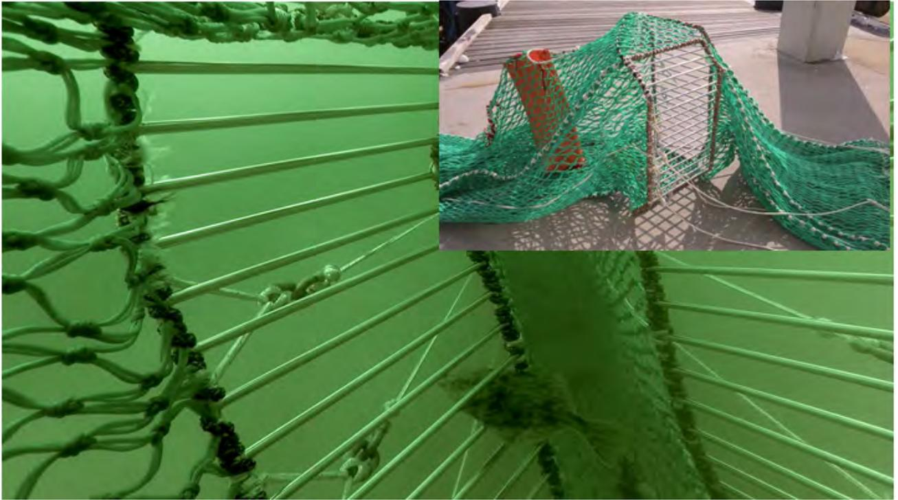
**Figure 1** Underwater recording of the *Freswind* during towing and a flounder escaping through the grid (canvas obstacle not shown here). Harbour picture showing the canvas obstacle (top-right).
