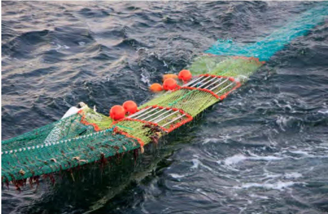
Figure 3.10. Hauling of the trawl with the first design of the grids device and the video recorder setup (white float).
